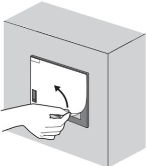
2) Peel the release paper off the back of the new protective sheet. With the protective film left on the sheet surface, attach the sheet on the GOT so that the USB environmental protection cover hole is just on the USB environmental protection cover of the GOT.
