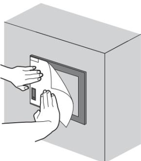
3) When attaching the protective sheet, make sure to fit the sheet on the GOT without leaving any clearance between the sheet and the GOT.
