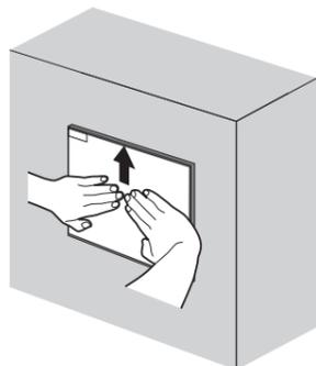
4) Remove the protective film from the protective sheet. When the user continues using the GOT with the protective film, the film may not be removed.
